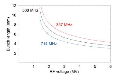
If the frequency is too low, the waveguide and cavities take up a lot of space. Also, it is convenient to use industry standard frequencies.
