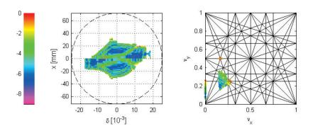
Depending on the details of the lattice design, the dynamic energy acceptance might be as small as 2%. Then, the Touschek lifetime with 0.75 mA bunch current would be only 16 hours.
