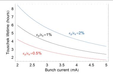
To keep a lifetime of more than 20 hours with 1% emittance ratio, the bunch current must be below 5 mA.
