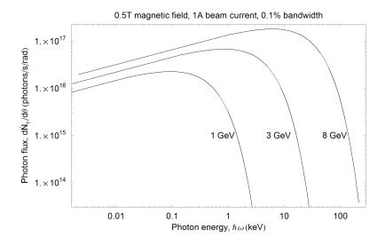
The flux of hard x-ray photons from a magnet with field strength of order  $0.5\,\mathrm{T}$  is substantially larger for beam energies above about  $3\,\mathrm{GeV}$ , compared with lower beam energies.
