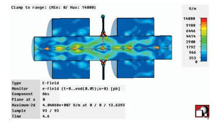
Wake fields can be short-range (acting over the length of a single bunch) or long-range (acting from one bunch to the following bunches), and can "kick" particles longitudinally or transversely.
