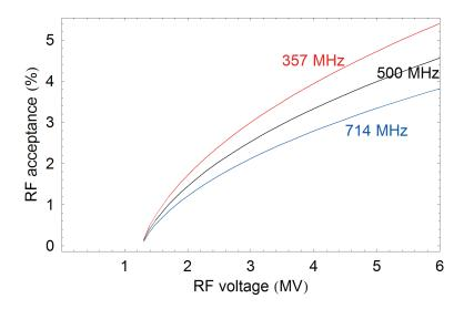
For a given rf voltage, reducing the rf frequency increases the rf acceptance.
