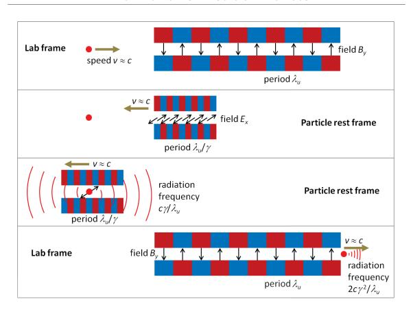
A detailed analysis of the undulator radiation gives the wavelength of the undulator radiation (observed along the axis of the undulator):
