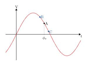
$\phi_s$  is the synchronous phase: this is the phase at which the rf cavities exactly replace the energy lost by synchrotron radiation:
