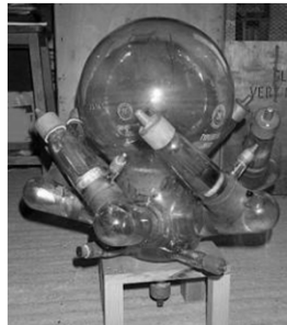
This is a 6-phase device, 150A rating with grid control. It measures 600mm high by 530mm diameter.
