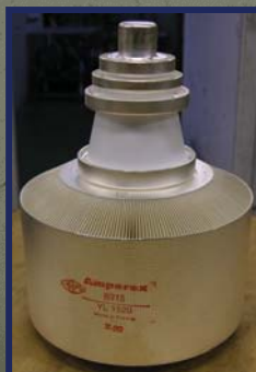
YL1520 (ex Philips, now Richardson), < 260 MHz, 25 kW
