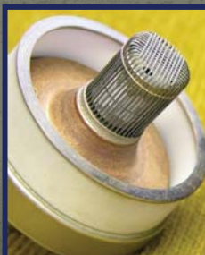
4CX250B (Eimac/CPI), < 500 MHz, 600 W (Anode removed)
