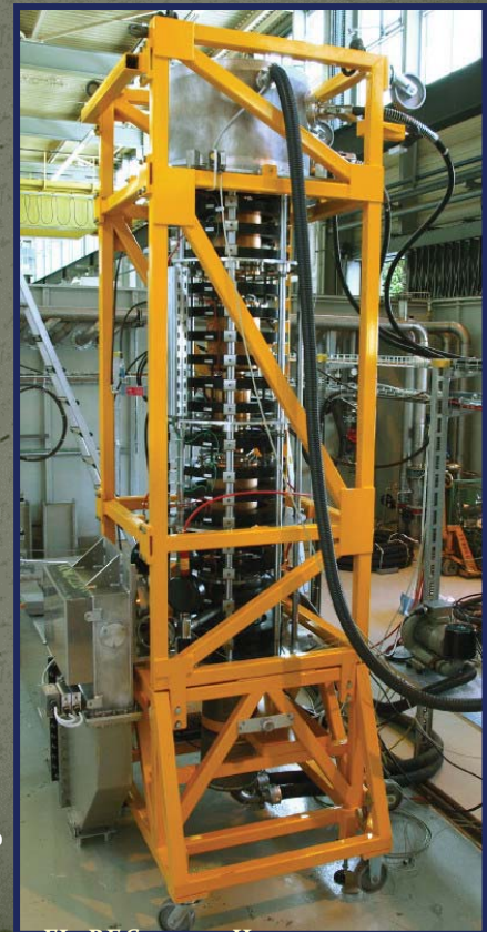
CERN LHC: 400 MHz, 300 kW, CW, \eta 62 %
