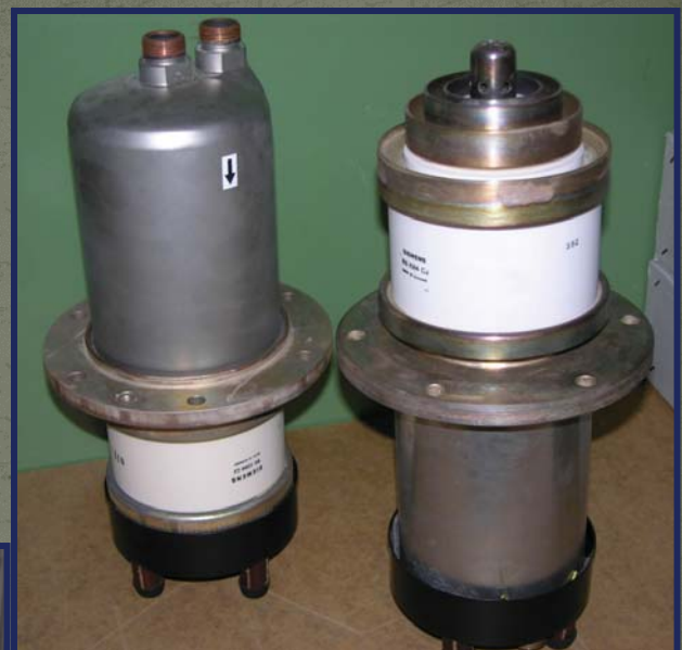
RS 1084 CJ (ex Siemens, now Thales), < 30 MHz, 75 kW
