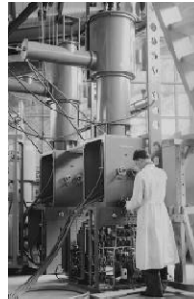
200 MHz triode amplifier (CERN Linac3)
