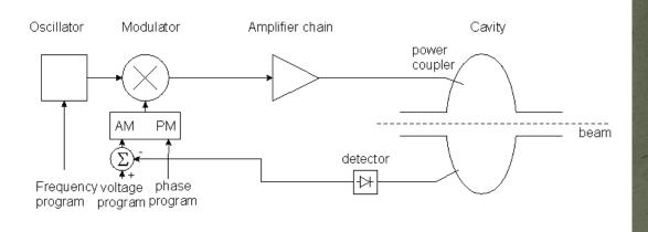
Compares the detected cavity voltage to the voltage program. The error signal serves to correct the amplitude
