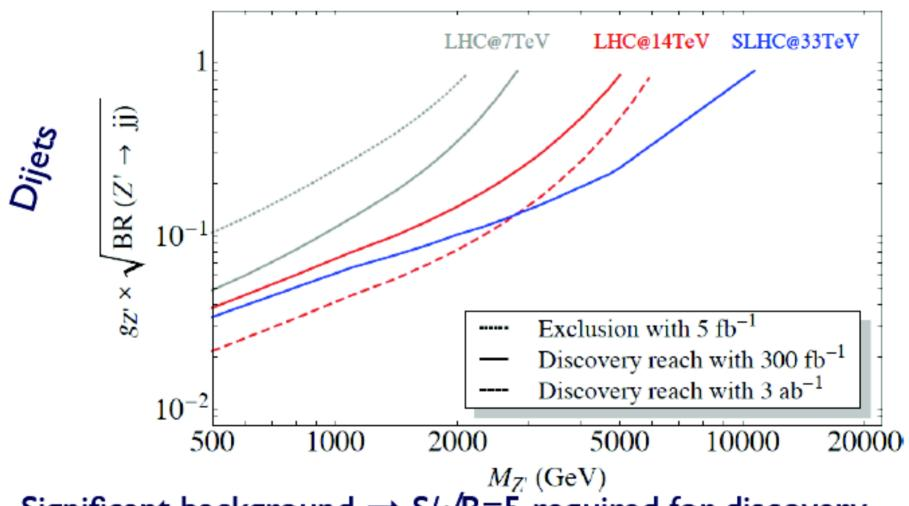
Significant background  $\rightarrow$  S/ $\sqrt{B}=5$  required for discovery, less than 3 for 95% C.L. exclusion
