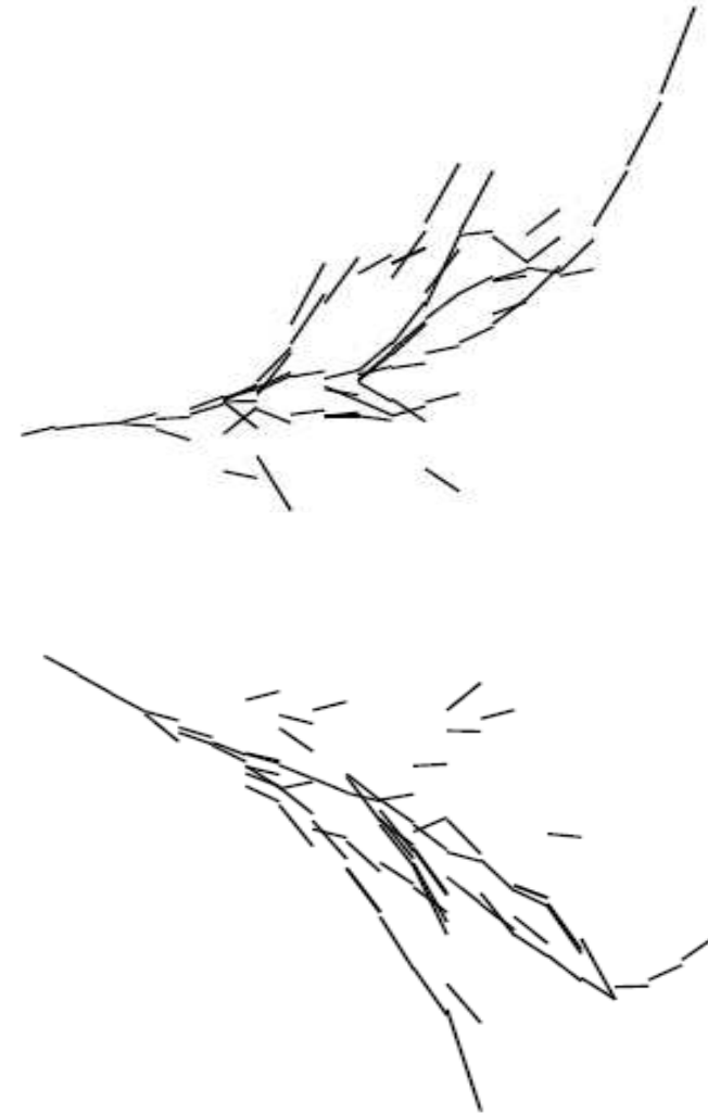
Figure 2. xz projection (left) and yz projection (right) of a reconstructed shower generated by a 6 GeV electron interacting in the \sim 3.3 X_0 ECC exposed at DESY. Each segment corresponds to a base-track associated with the reconstructed electromagnetic shower.
