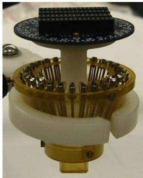
28 tetrodes with microdrives (Neuralynx)
