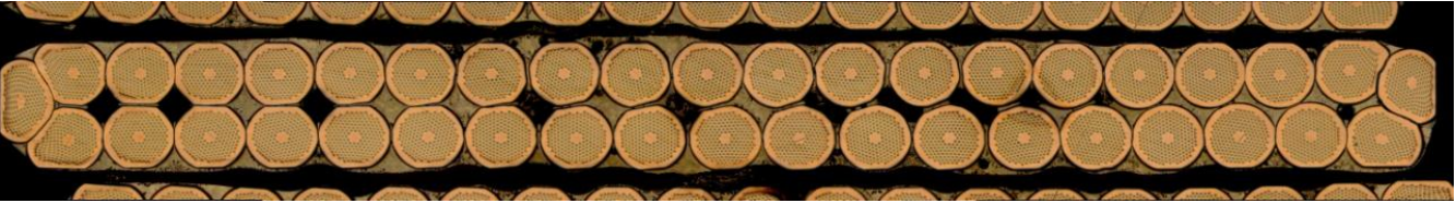
Width of 20.9 mm Total compaction 87.5 %
