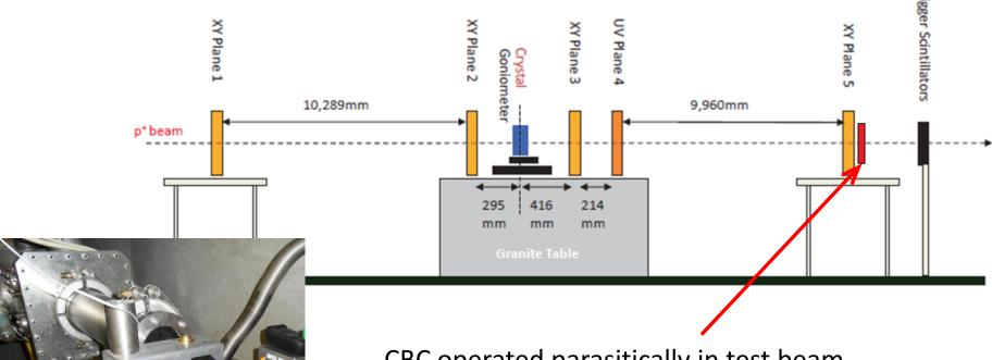
CBC operated parasitically in test beam (using sensor of ~134 µm pitch)
