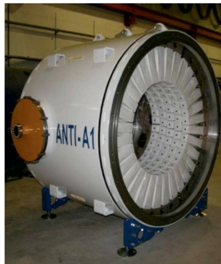
A LAV station constructed at Frascati
