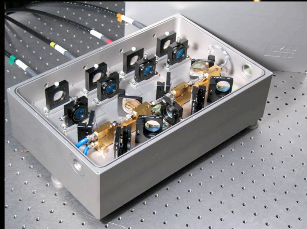
35W CW output 1.06um laser amplifier (Enhanced LIGO)
