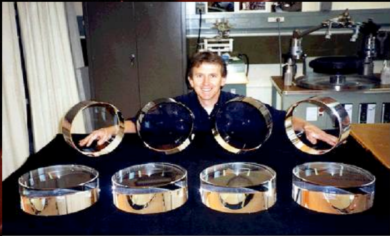
Initial LIGO fused silica optics
