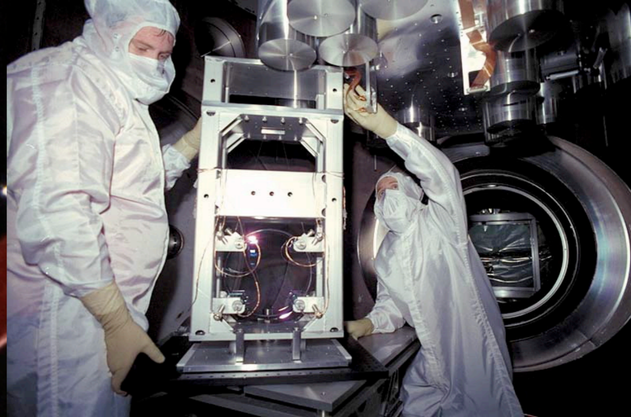
Livingston beam splitter installation
