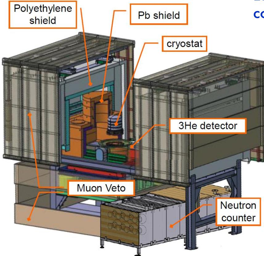
Shielding: 4800mwe rock; 20cm lead; 50cm polyethylene
