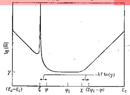
Dependence of critical concentration of recombination centers on the recombination center energy (cross sections are fixed and defined in  $\gamma$ )
