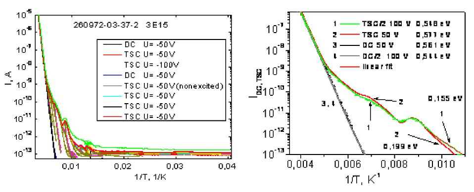
The dark current and TSC dependence on temperature at different bias. Left – the same, a wide T range. The sample number, irradiation fluence neutrons/cm<sup>-2</sup>, bias voltage and activation energy are given in the inset.
