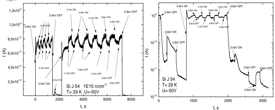
An evidence of a double role: excitation of PC and quenching of photoresponse. Si excited by 0.9 eV light, additional extrinsic excitation.
