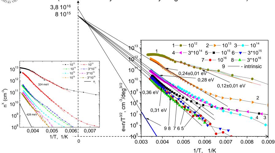
Electron concentration (a) and thermal excitation rate (b) dependence on temperature.
