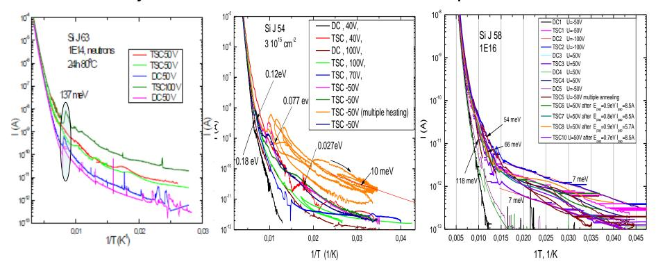
The dark current and TSC dependence on temperature at different bias in the irradiated by neutrons Si samples.
