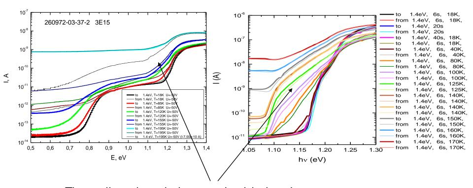
Thermally activated photoconductivity band (left – measurements in p-i-n structure)
