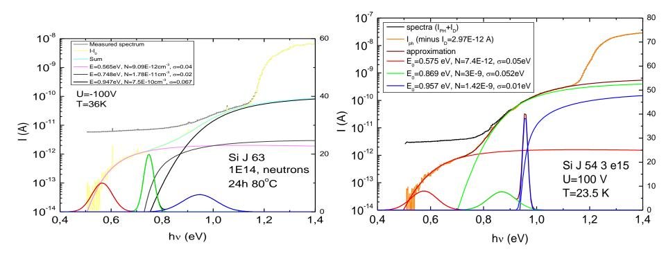
The PC with a background excitation allows to reveal the centers near to the midgap that probably are most important for the generation current.
