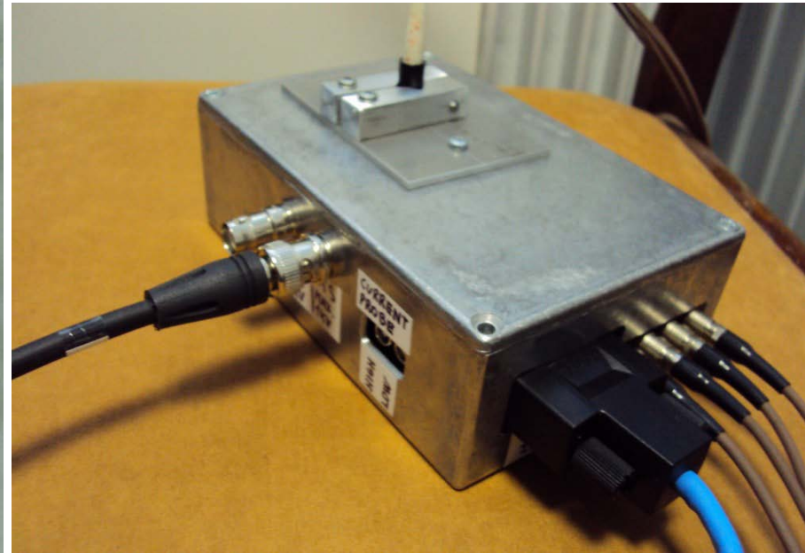
Box with preamplifier and detector, black cable in front is high voltage supply, RS232 connector is low voltage supply, four data cables on right are connected to the Evaluation board, on the top it is optical fibre
