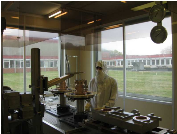
Fig. 4: coupler assembly in the class 10 clean room
