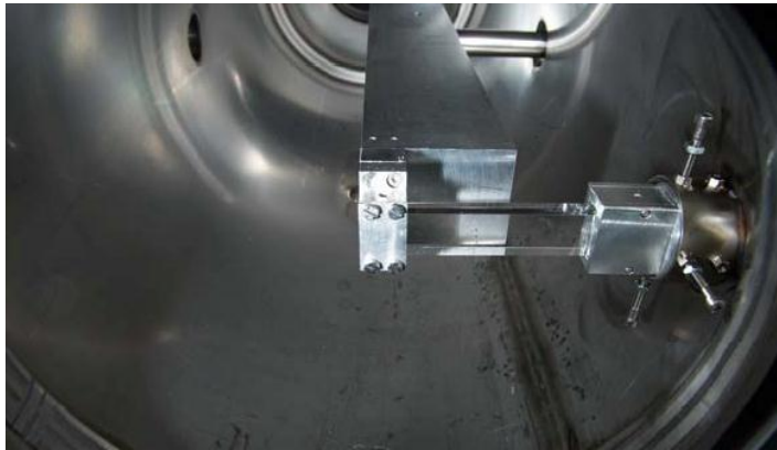
TAL absorber & Quartz Cerenkov detector
