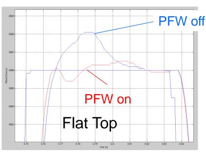
The RST algorithm is tuned with PFW. No active compensation is introduced in the control. If PFW are switched off the behavior is worst because the internal dynamic of the Bfield regulator is not high enough
