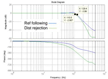
RST regulator with FFW to compensate for converters voltage drops. Executed in P80. *Tsampl=1ms*. Each polynomial has a maximum of 10 coeffs for a total of 30.
