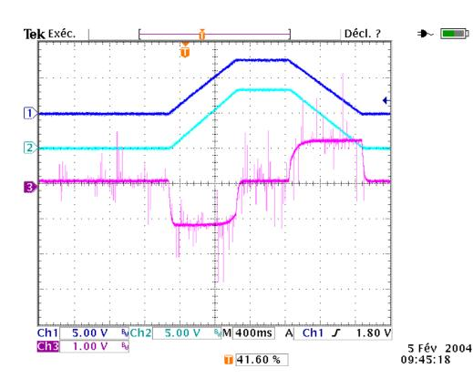
The main dipole current rises from 0 to 5kA with 6500 A/s dynamic
