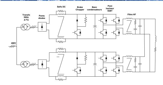
2 IGBT bridges connecte in parallel for the B8
