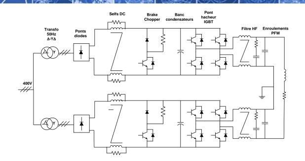
2 IGBT bridges connecte in series for PFW circuits
