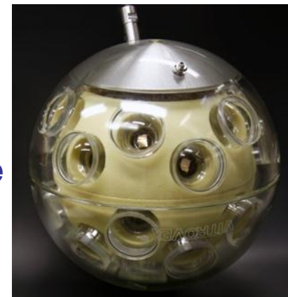
KM3NeT: 31 3" PMTs in 17" sphere
