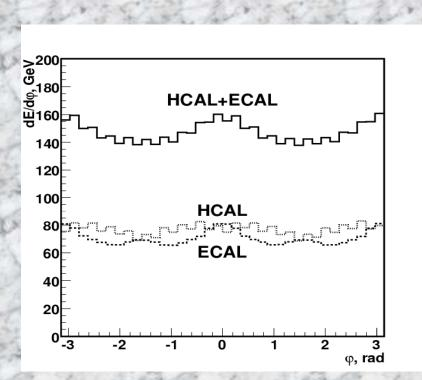
Azimuthal E<sub>T</sub> distribution in different calorimeter layers
