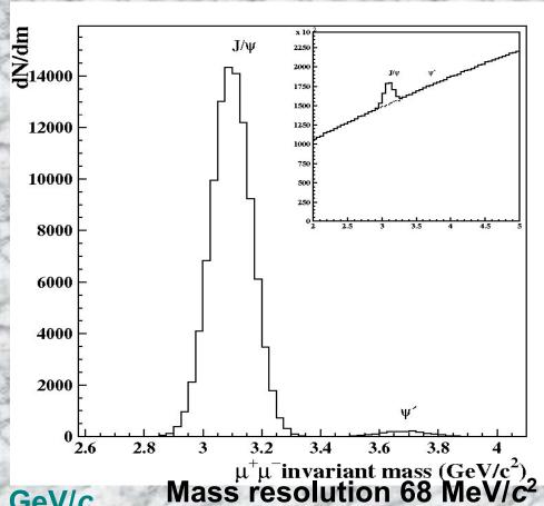
full reconstruction, p<sub>T</sub> cut 1.5 GeV/c Mass resolution 68 MeV/c<sup>2</sup> ~100k J/ψ per month, tagging method full reconstruction, p<sub>T</sub> cut 3 GeV/c
