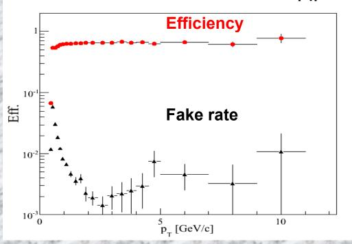
For p<sub>T</sub>: 1 - 10 GeV/c: efficiency ~ 70 %, fake rate ~ 1% Momentum resolution ~ 3% (2% - barrel, 4-5% end-caps)
