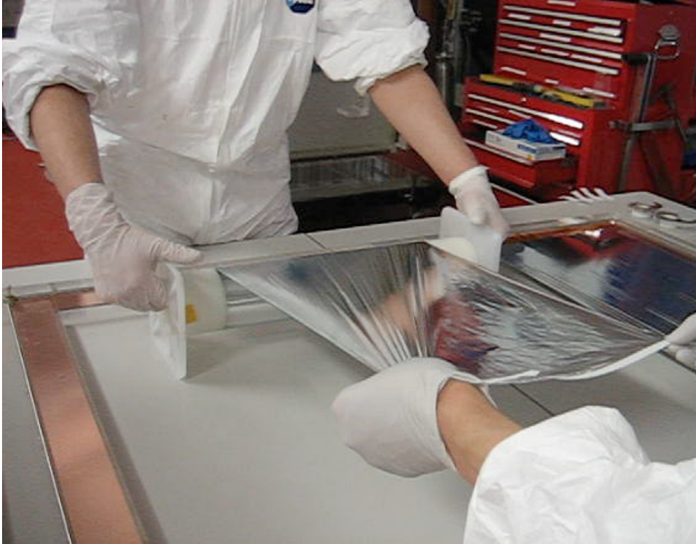
Thin film cathode construction underground
