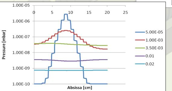
Calculated with thermal analogy model (and Monte-Carlo model)
