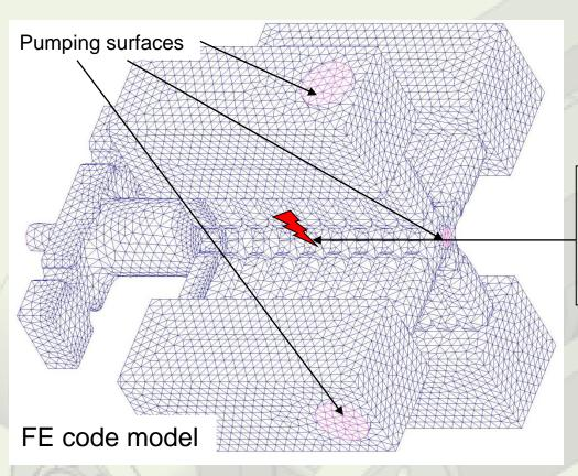
2.10<sup>12</sup> H<sub>2</sub> or CO molecules released during breakdown (in a baked system)
