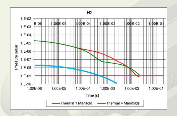
Pressure goes to < 10<sup>-9</sup> mbar in less than 1 msec! This is faster than the sampling time of common vacuum gauges...
