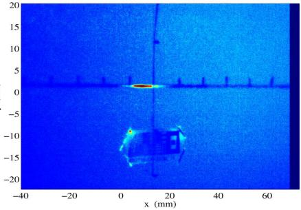
Profile image of LCLS beam successfully extracted into line upstream ESA, ready for **CLIC studies**.
