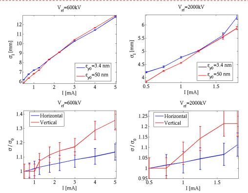
Top: Bunch length versus current for low (blue) and large (red) vertical emittance for Vrf=600kV (left) and Vrf=2000kV (right) Bottom: The IBS effect on the horizontal (red) and vertical (blue) beam size.
