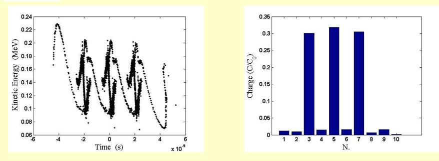
Longitudinal phase space after sub-harmonic bunching Same total gap-voltage but fewer cells (2 instead of 6) 35-39 KV needed
