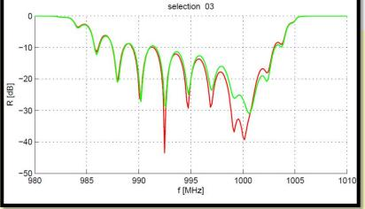
**Input and output coupler design finished** Correct match, input reflection < 30 dB. (red and green: two different geometries; red is final)
