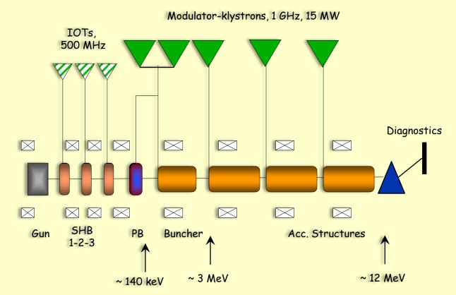
Gun, sub-harmonic bunching, bunching, three accelerating structures, 5 long pulse klystrons and modulators, diagnostics
