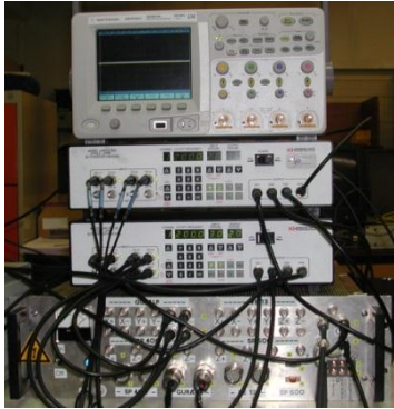
Amplifiers, filters input/output board for signal conditioning
