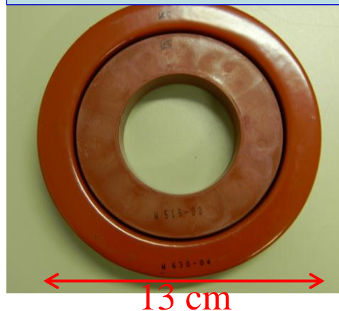
Sample transformer cores
