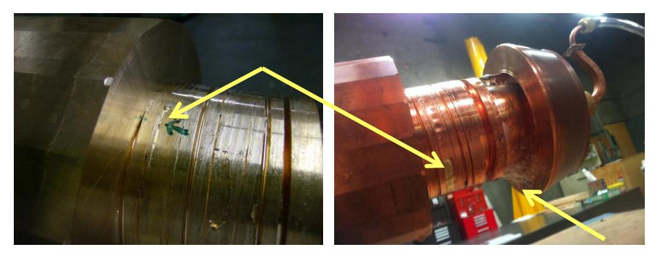
Tube walls thinned to 0.030" in places when mandrel prepped for jaw braze Repaired with "CuSil"
