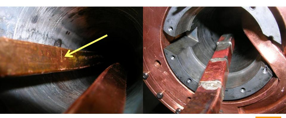
Suspect weakening in non-OFE Cu tubing at crystal grain boundaries after last of many high temperature firings Repaired with solder patch
