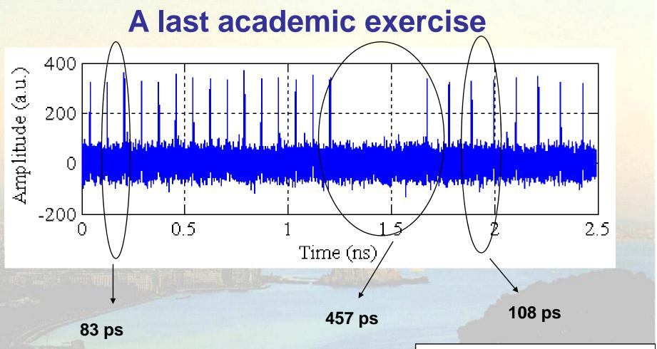
RMS bunch length = 13.3ps Train duration = 2.5ns Nb of bunches = 23 Peak current = 293A
