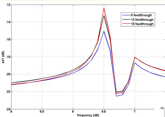
In order to reduce this enhancement, would have to happen that the distance between two feedthrough's should be at least equal to one half of the resonant mode wavelength
