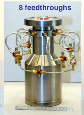
The existing design is based on a previous design for the CTF2 (63 MHz ≤ bandwidth ≤ 10 GHz )
