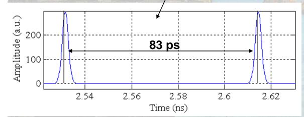
Bunch separation = 83ps RMS bunch length = 13.3ps Train duration = 8.3ns Nb of bunches = 100 Peak current = 293A
