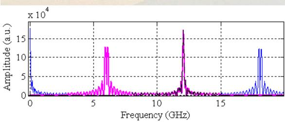
Because of the different, larger, bunch spacing, in the spectrum some new peaks appear at lower frequencies
