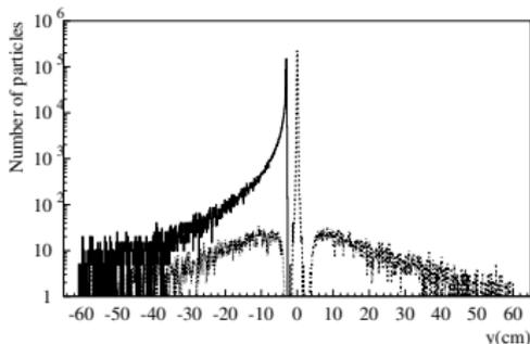
Vertical beam profiles at the exit of the fourth extraction magnet (35 m from the IP).
