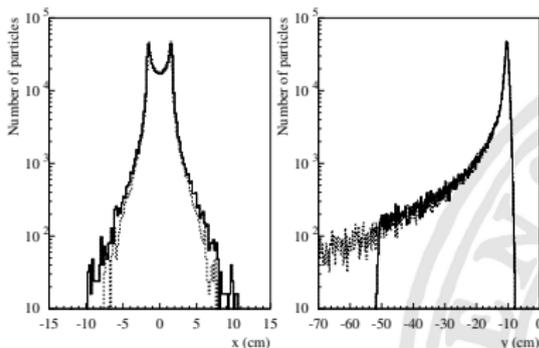
The transport of the photons remains loss free from the IP to the dump, where  $\sigma_x(\gamma) = 8.2$  mm and  $\sigma_y(\gamma) = 6.5$  mm.
