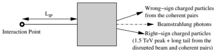
For 1.5 TeV particles, the vertical deviation must be 10 times larger than the worse photon cone size at the last dipole exit [ $\text{rms}^\gamma(y') = 80 \mu\text{rad}$ , with an offset at the IP].
