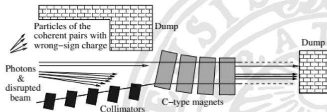
Charged particles with  $\delta < -0.85$  are absorbed in five 1 m long collimators. Loss free transport through four C-type magnets.
