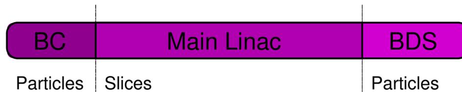
⇒ PLACET can simulate: bunch compressor, main linac, drive beam, beam delivery system (including crab cavities and instrumentation), interaction point (using **guinea-pig**) and soon : post collision line
