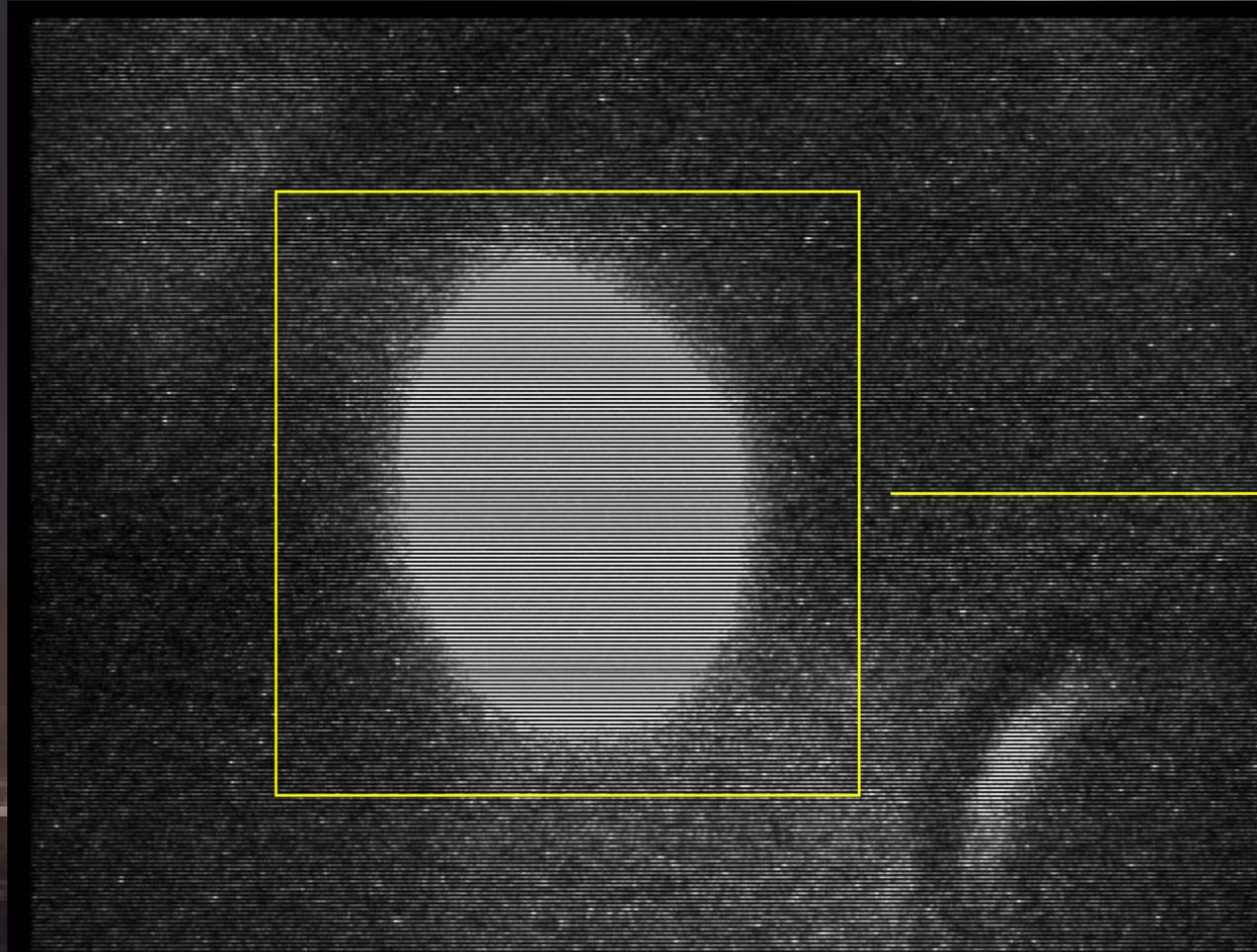
A LabView program calculates the average pixel intensity for each frame and triggers above a variable threshold...
