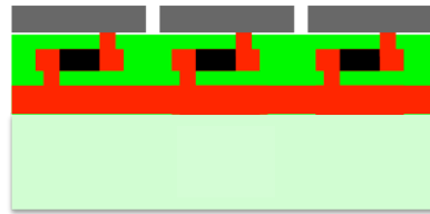
Buried resistors “BR” connect strips to resistive pads
