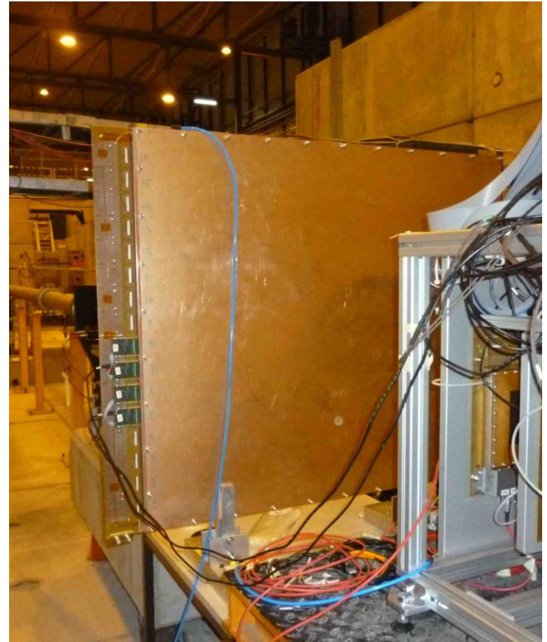
1 x 1 m 2 MM in H6 test beam
