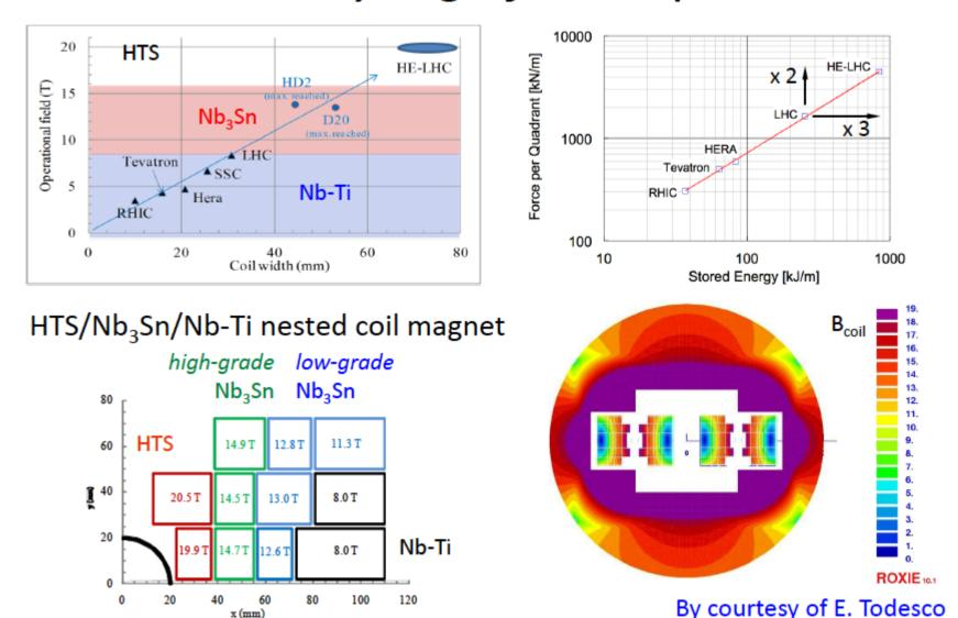
Aim is to double the B-field using High-critical Temperature Superconductors to allow twice the beam energy. It is in practice a new accelerator
