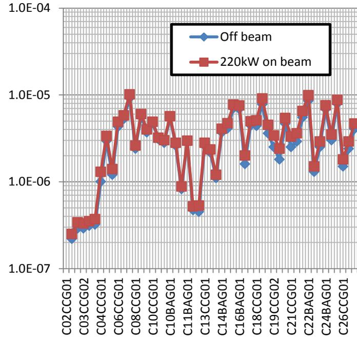
There is a conditioning effect by the beam during a continuous beam operation.
