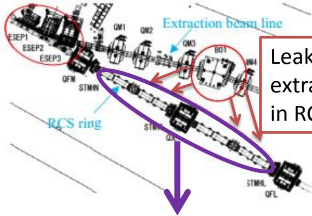
Leakage field from a magnet in the extraction line distort the beam orbit in RCS.
