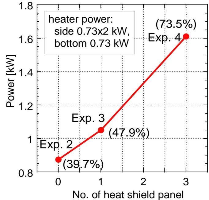
Required heater power to reach a kicker temperature up to 100 °C.
