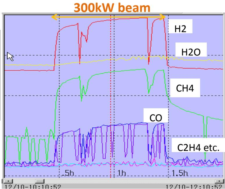
Especially in the beam operation just after a maintenance, we see the large pressure increase.
