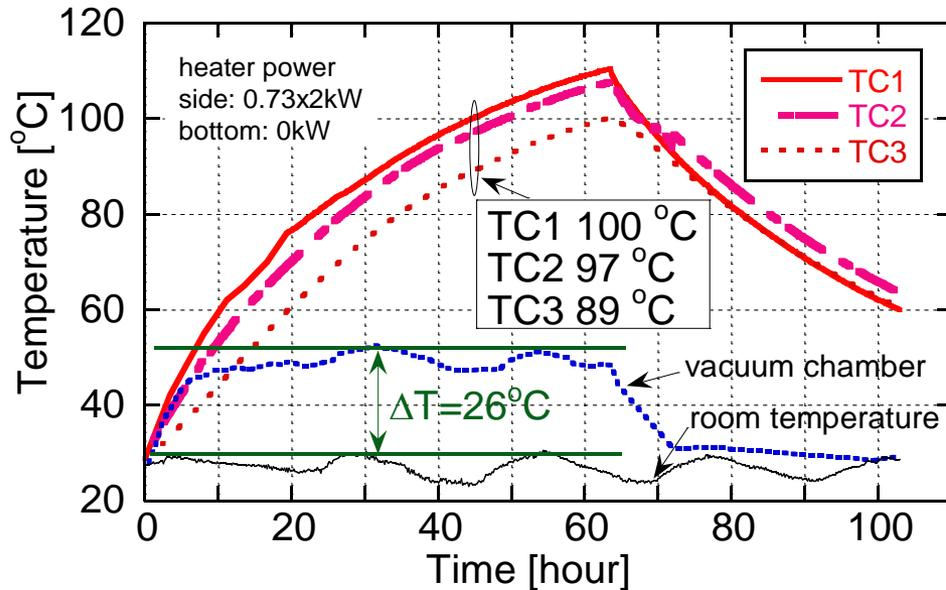
Temperature of ferrite cores and vacuum chamber.
