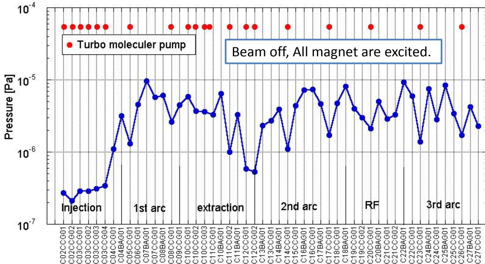
Pressure of less than  $10^{-5}$  Pa is stably maintained.
