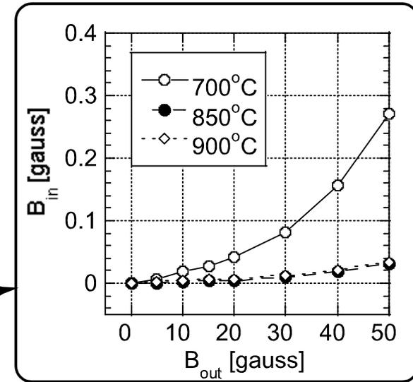
Good shielding characteristic for the annealing temperature with more than 850 degC(10H).
