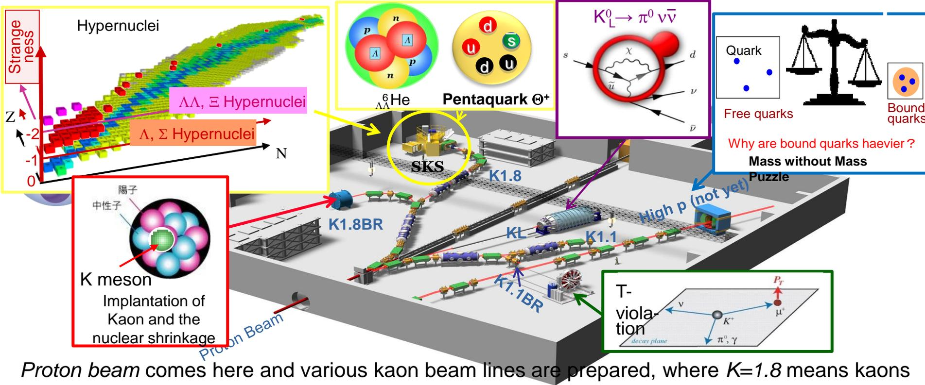
Proton beam comes here and various kaon beam lines are prepared, where  $K=1.8$  means kaons with momentum of  $1.8 \text{ GeV}/c$ .
