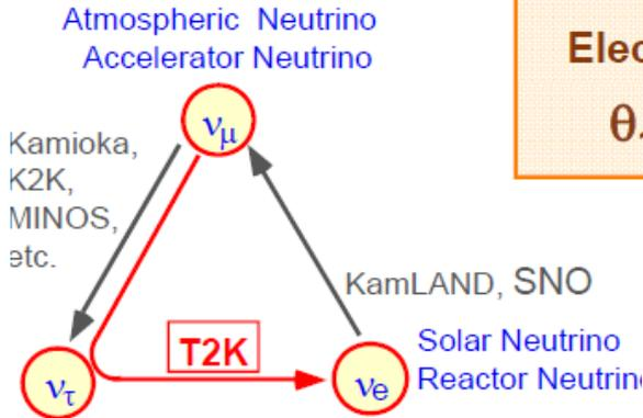
Muon neutrino beam is produced at J-PARC with 2.5 degrees off from the direction to the Super-Kamiokande (SK), travels 295 km across the earth, and is detected by SK.
