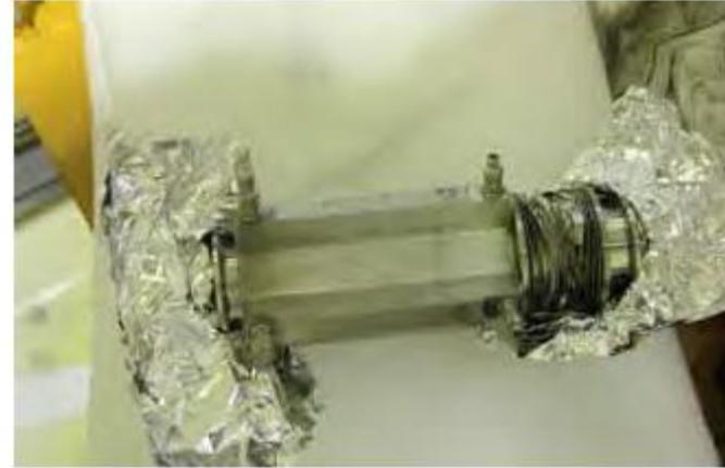
BPM (Beam Profile Monitor) extracted from Q-Magnet. Bellow was destroyed.
