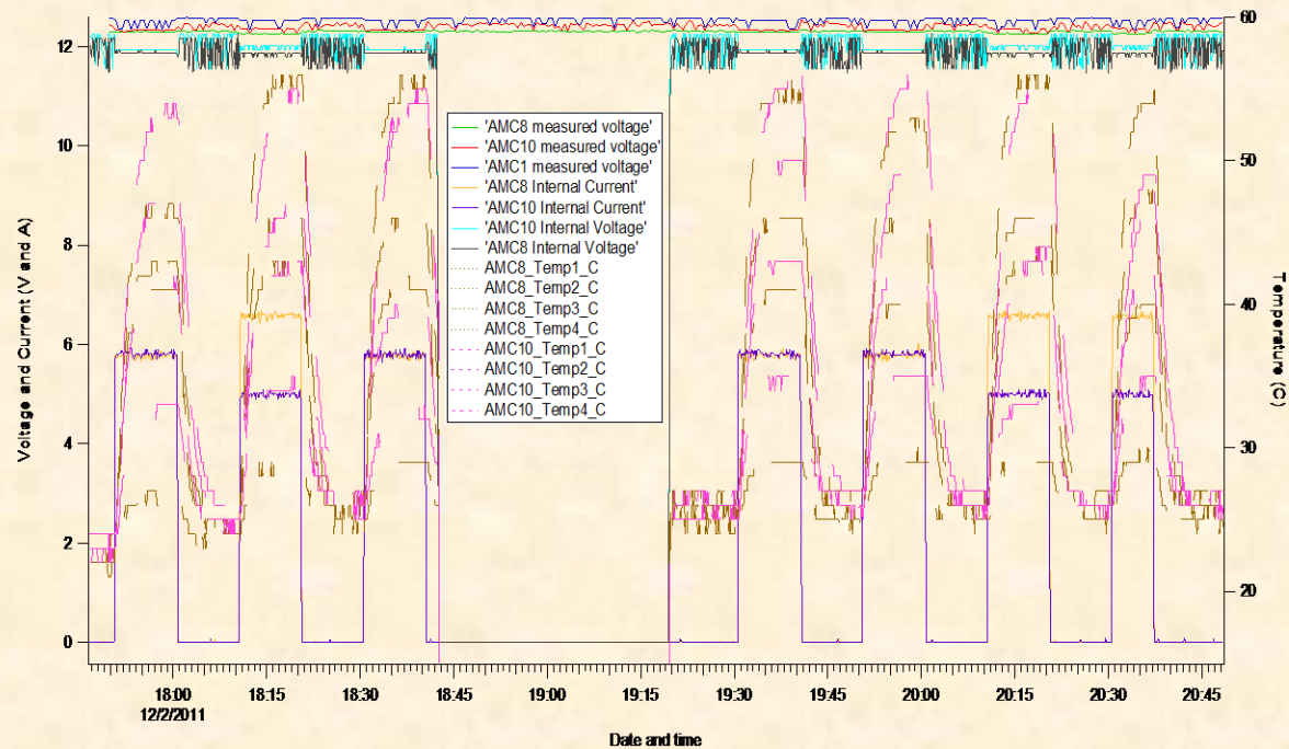
Long term measurements with load variations and temperature monitoring
