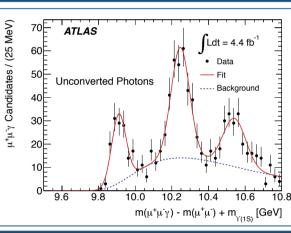
The  $m(\mu^+\mu^-\gamma) - m(\mu^+\mu^-) + m(Y(1S))$  distribution of  $\chi_b \rightarrow Y(1S) \gamma$  candidates reconstructed from unconverted photons.
