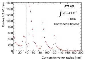
The distribution of conversion vertex radius from the beam axis. The four peaks correspond to the beam pipe and the inner three silicon detector layers. To reduce combinatorial background, conversion candidates are required to be reconstructed with R > 40 mm.
