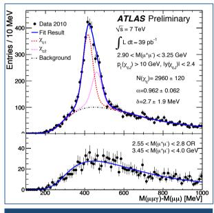
The  $m(\mu^+\mu^-\gamma) - m(\mu^+\mu^-)$  distribution for selected  $\chi_c$  candidates with photons reconstructed from direct calorimetric measurements alone.
