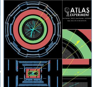
An event containing a candidate  $\chi_b$  (3P)  $\rightarrow$ Y (1S)  $\gamma$  decay. The photon is reconstructed with a direct calorimetric measurement. For this candidate,  $m(\mu^+\mu^-\gamma) - m(\mu^+\mu^-) + m(Y(1S)) = 10.54$  GeV.
