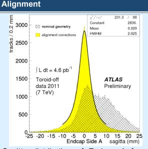
Sagitta distribution of Endcap A from "Nominal geometry" and "after alignment corrections". Multiple scattering is the dominant contribution for the width after the corrections. We observe mean values of +29µm ± 12µm. Similar correction was done for Endcap Side C.
