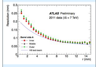
Spatial resolution as a function of the radius measured separately for Inner (red squares), Middle (black triangles), Outer (green triangles) chambers of the Muon Spectrometer Barrel side A on the top and Endcap side A on the bottom.
