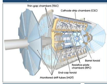
Left: The muon system of the ATLAS detector consists of
