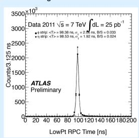
RPC timing Resolution for clusters matched ( $|\Delta\eta|$ ,  $|\Delta\phi|$  <0.1) to combined muons was measured to be from 1.9 ns to 2.1 ns after the offline calibration.
