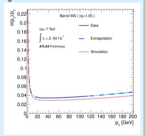
Muon Spectrometer momentum resolution for Barrel.
