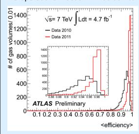
The plot shows the distribution of the measured 2010 and 2011 RPC gas volume efficiencies. The improvement mainly comes from High Voltage working point correction and better control of the gas flux.
