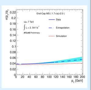
Muon Spectrometer momentum resolution for Endcap.
