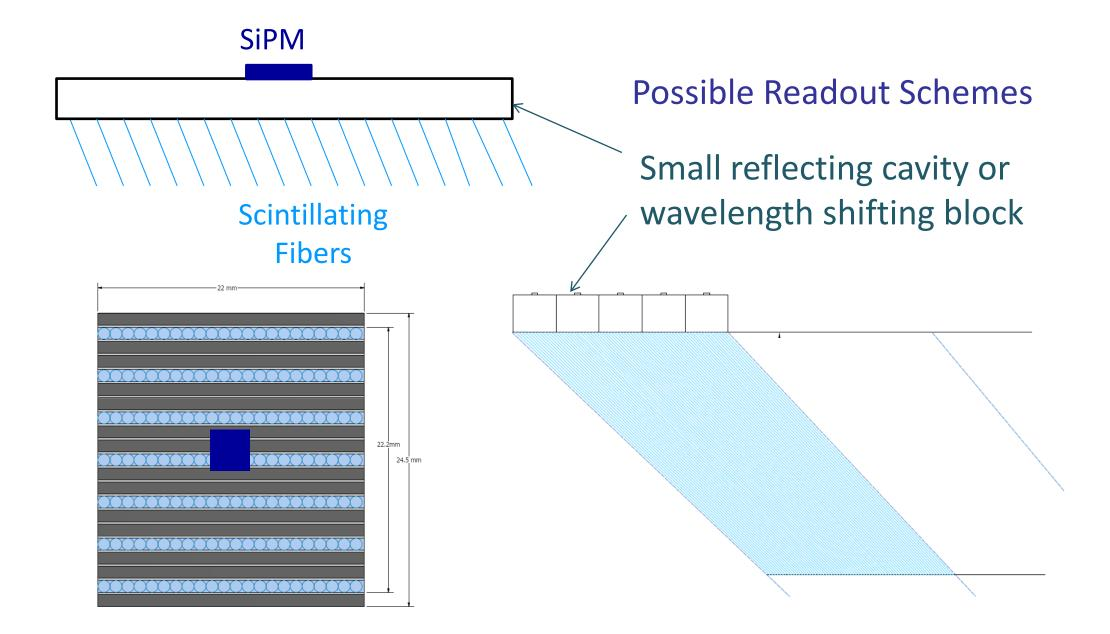
Need to match ~150 1 mm diameter fibers onto a single 3x3 mm<sup>2</sup> SiPM with good efficiency and uniformity ( $\varepsilon_{area} \sim 2\%$ )
