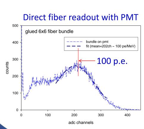
With a sampling fraction of 4%, 100 p.e./MeV in scintillator (direct readout with PMT)  $\Rightarrow$  4000 p.e./GeV of energy deposit in the calorimeter
