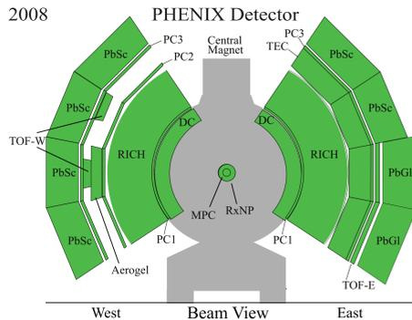
Figure 1: PHENIX detector configuration 2008
