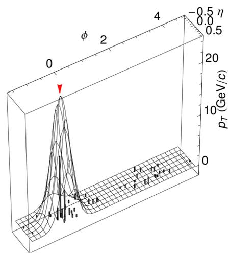
Figure 2: Example of Gaussian filter local maximum finding
