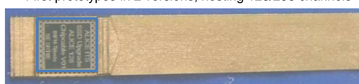
First microcable prototype with 42.5 \mu\text{m} inter-trace pitch (SE SRTIE - Kharkov, UA)
