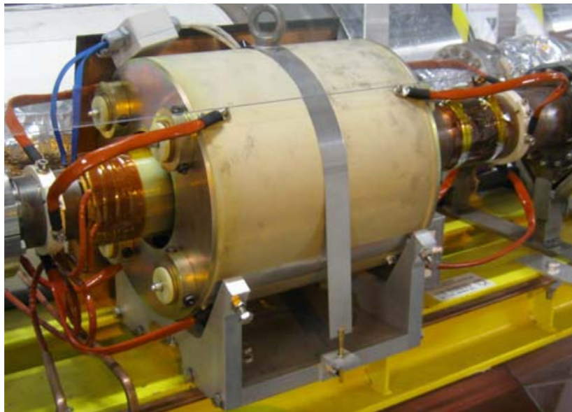
DCCT - DC Current Transformer accurate, but measures everything
