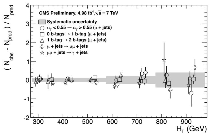
Systematic uncertainties on MC ratios are determined from detailed closure tests using various control samples from data to validate relative contribution of various backgrounds, kinematic properties & b-jet reconstruction.
