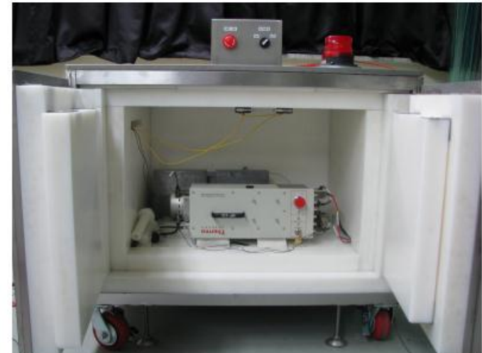
Figure 3.17: Neutron generator inside the shielding box
