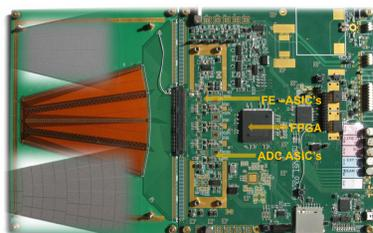
FE ASIC comprises 2 feedback technologies (4 channels each per chip). The number of assembled channels was 32, 8 channels were additionally readout by a CAEN ADC. FE can be operated in 2 modes for physics and calibration measurements. GaAs:Cr sensors were previously tested for radiation hardness in an electron beam up to 1.5 MGy.
