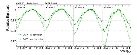
Reconstructed energy as a function of the local position of the most energetic crystal in the cluster, with E/p method.
