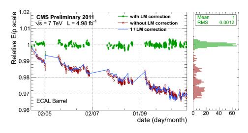
Stability of the energy scale after monitoring corrections with Wev events.
