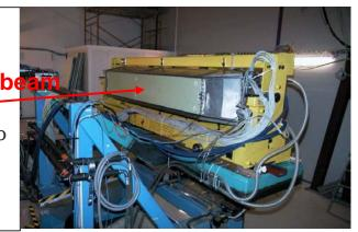
Channel intercalibration with cosmic muons (only Barrel SMs)
