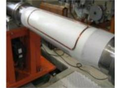
TiN-coated beam pipe with antechambers
