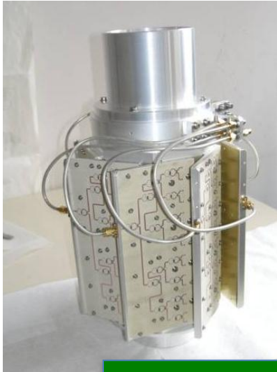
Slot-coupler RF structure (by IKP FZJ)
