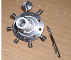
wet turboexpander (300 000 turns/min)
