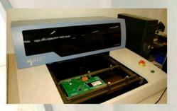
DIGITAL OPTICAL INSPECTION - Digital optical inspection machine (AOI) of last generation, brand Mirtec, for the thorough inspection and extreme precision of SMD components, before and after assembly, so that we can ensure high quality and reliability.
