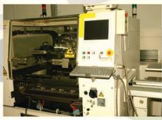
**PICK & PLACE JUKI FM 760,** with a capacity of assembling 760-7500 cph with laser alignment and vision system for BGA and uBGA placement. Capability of placing 0402 - 50x50sqmm and equipped with MTC (Multi Tray Feeder).
