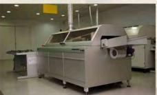
DIP SOLDERING - Wave soldering machine, brand Inertec, composed of area for refinishing spray, 3-zone preheat and wave solder turbulent (last generation). This equipment is properly equipped with 10 transportation vehicles and is already prepared for welding in accordance with the RoHS standard, raw material and component solder without lead.
