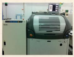
**Screen Printer DEK Horizon 03iX** – Automatic solder paste printing for SMT technology, machine alignment /capapbility; 2 Cpk @ +/- 12.5um, 6 sigma, process alignment / capapbility; 2 Cpk @ +/- 25um, 6 sigma, cycle core time 12 secs; maximum print area; 510mm (X) x 508.5mm (Y). Stencil cleaning is fully programmable.
