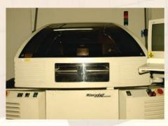
**SCREEN PRINTER MPM UP3000** - Automatic solder paste printing for SMT technology with dispenser folder, alignment of the screen by camera and 2D inspection.
