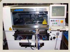
PICK & PLACE JUKI 2060, can place a wide range of components from 0201 and ICs to odd-form, all at a high rate of speed, 12,500CPH, increasing production rates.
