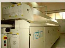
REHM OVEN, composed of six zones, five heating and cooling, transport chain, allowing the production of double-sided, with 5, 5 meters long, lower support for the hardware of higher dimensions. This oven is ready to use nitrogen.
